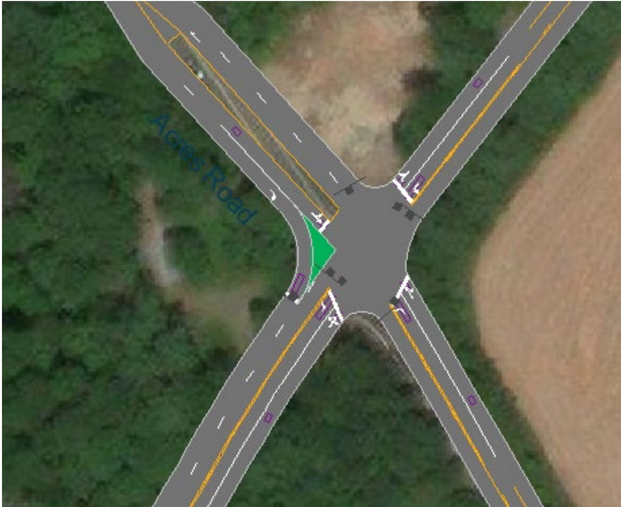
Figure 4.1 – Bakertown Road/Acres Road Slip Ramp Alternative
