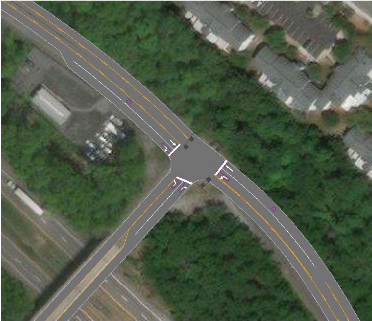
Figure 4.9 –Forest Avenue/ Schunnemunk Road Signal with Turn Lanes
